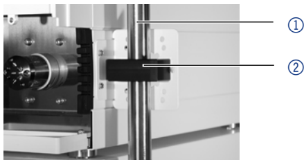
Fig. 16 Fully mounted sample loop front view
