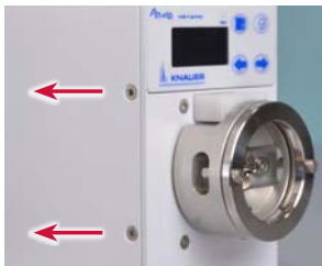
Fig. 18 VU 4.1 removing screws
