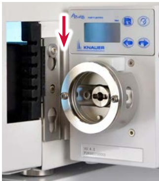
Fig. 23 Lock with lower screw
