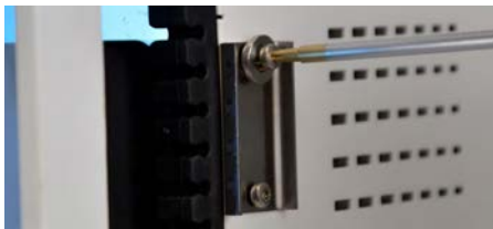
Fig. 33 Guidance clamp on AZURA® L device
