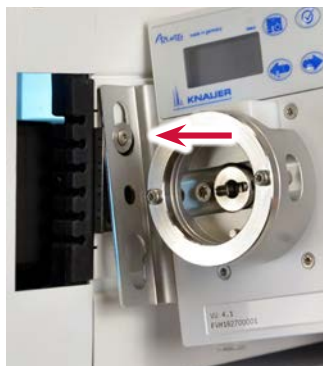
Fig. 28 Put keyhole on washer (exemplary picture with VU 4.1)
