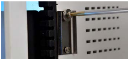
Fig. 27 Guidance clamp on AZURA® L device
