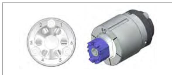
Fig. 14 Correct orientation of the direct sampling valve with ports 1, 2 and the chocking groove at the top
