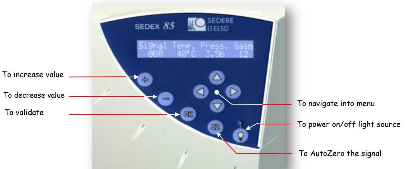
Figure 3-1: The Control Panel
