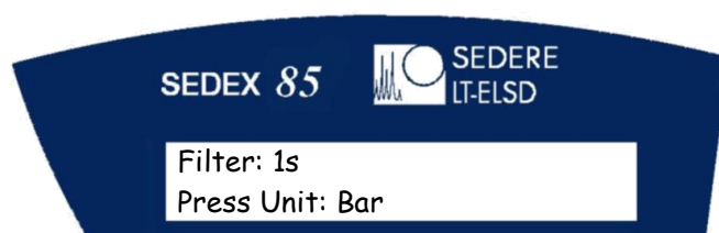
Figure 3-6: The Noise Filter/Pressure Unit Screen
