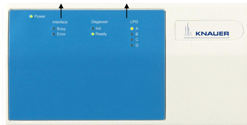
Figure 8 Front view of Smartline Manager with Degasser LED's
